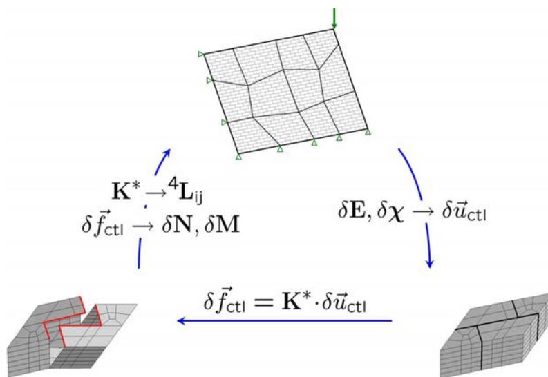
Fig. 12. FE<sup>2</sup> computational scheme for shell structures.
