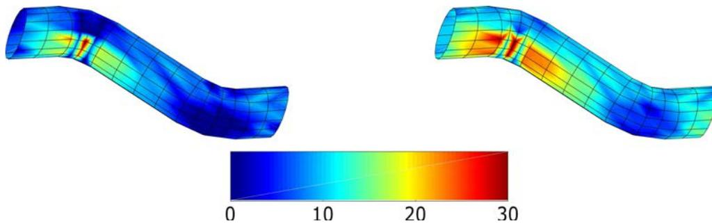
**Fig. 6.** Unit cell composed of four plain weave plies – Stress state at the warp yarns – matrix interface for in-plane tension along the warp direction combined with bending: (left) normal (peeling) stress  $\sigma_{nn}$ , (right) delamination stress defined by (16) with  $\alpha = 0.5$ .
