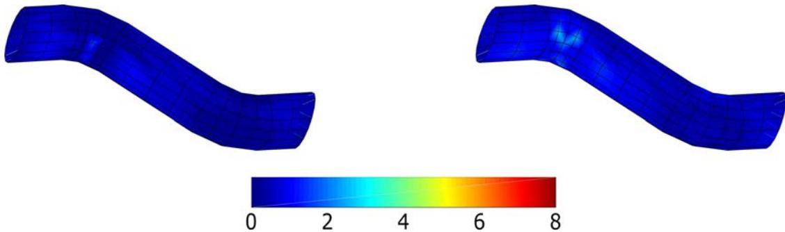
**Fig. 4.** Stress state at the warp yarns - matrix interface for in-plane tension along the warp direction: (left) normal (peeling) stress  $\sigma_{nn}$ , (right) delamination stress defined by (16) with  $\alpha = 0.5$ . The colorbar is adapted to ease the comparison with Fig. 5.
