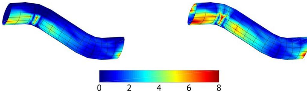
**Fig. 5.** Stress state at the warp yarns – matrix interface for in-plane tension along the warp direction combined with bending: (left) normal (peeling) stress  $\sigma_{nn}$ , (right) delamination stress defined by (16) with  $\alpha = 0.5$ .
