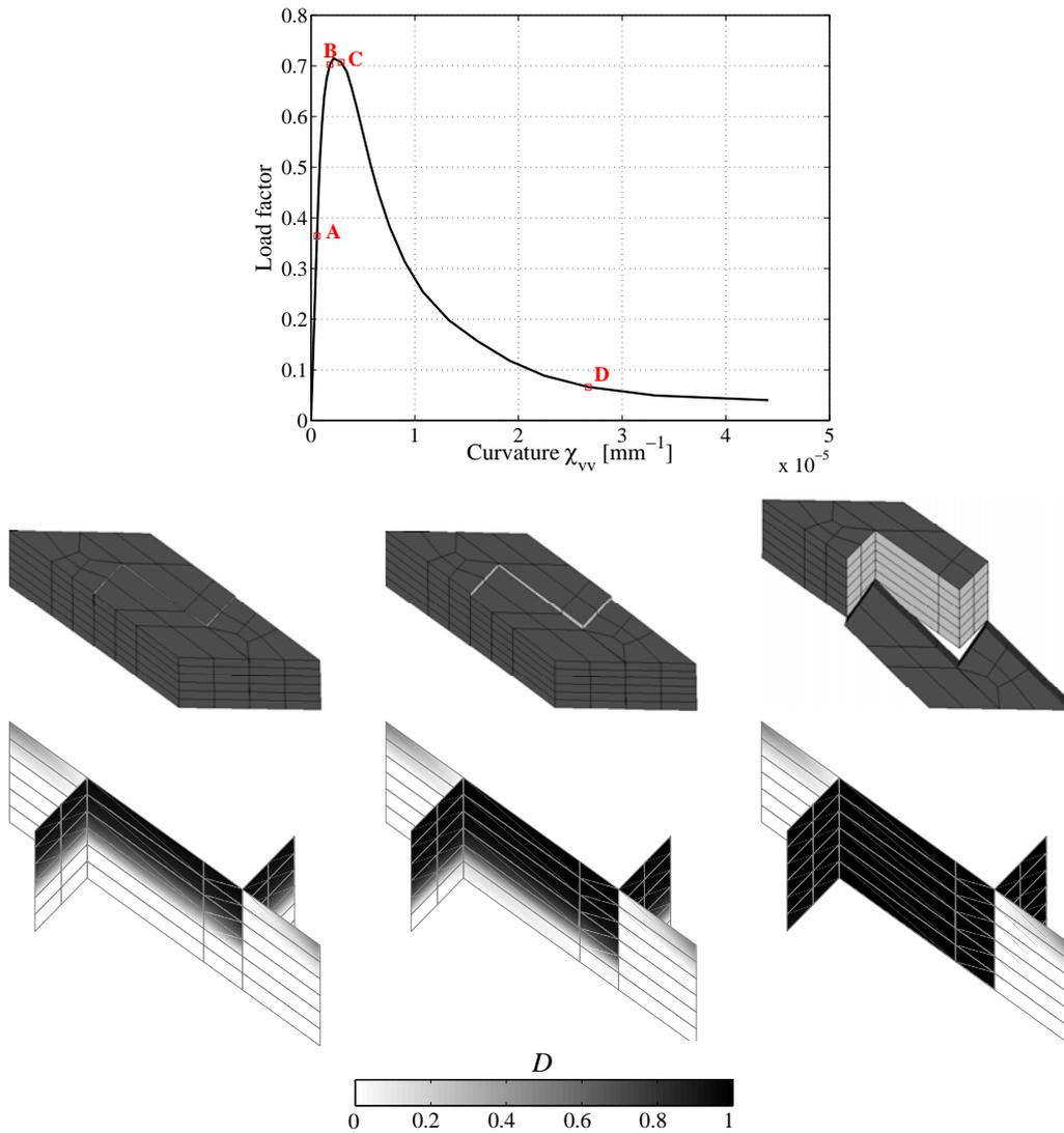
**Fig. 9.** Global response of the unit cell subjected to bending with stair-case crack opening. The amplified deformed shape and the damage states are illustrated for states B (left), C (center) and D (right) of the response curve.
