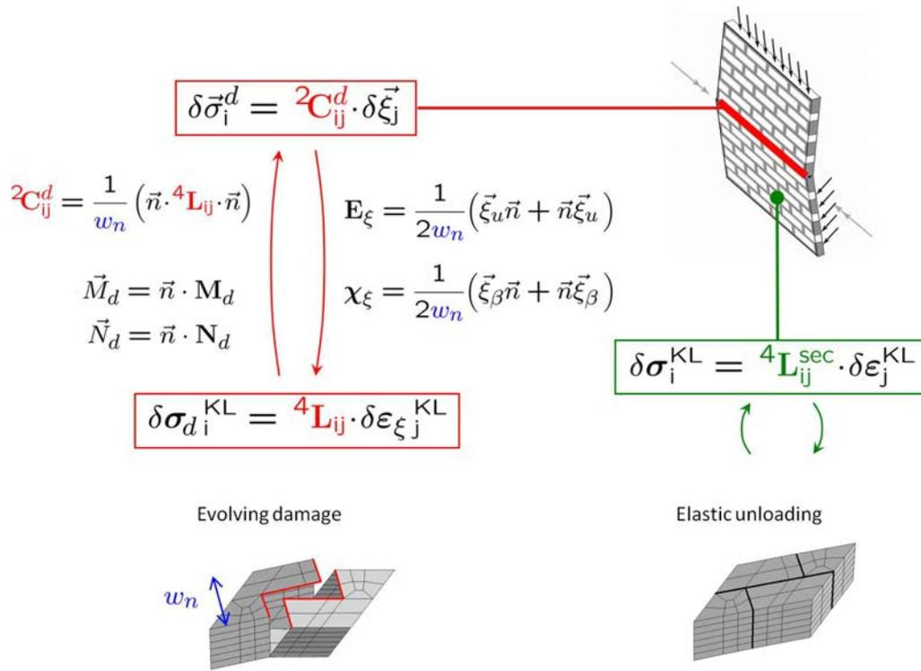
Fig. 13. Localisation-enhanced  $FE^2$  computational scheme for shell structures.
