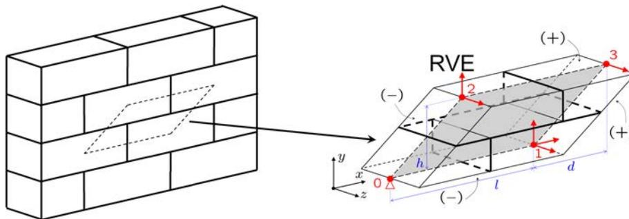
**Fig. 7.** Through-thickness RVE for running bond masonry [35].
