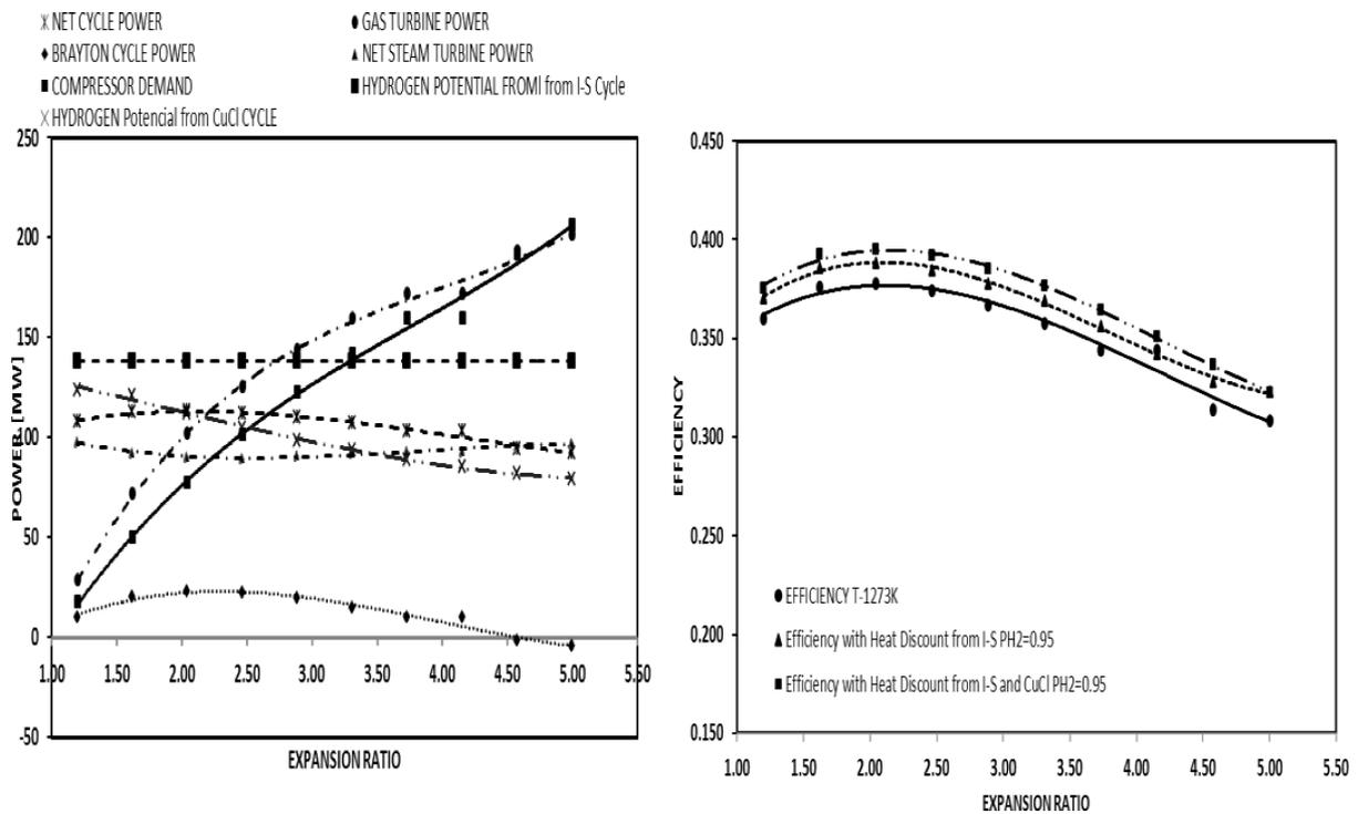
Fig. 8. Thermal power and thermal efficiency at two different outlet reactor temperatures:  $T = 1073$  K and  $T = 1273$  K for the case with hydrogen production using I-S cycle in which the amount of power dedicated to the production of hydrogen is equal to 30 MW for I-S cycle and 27 MW for Cu-Cl cycle.
