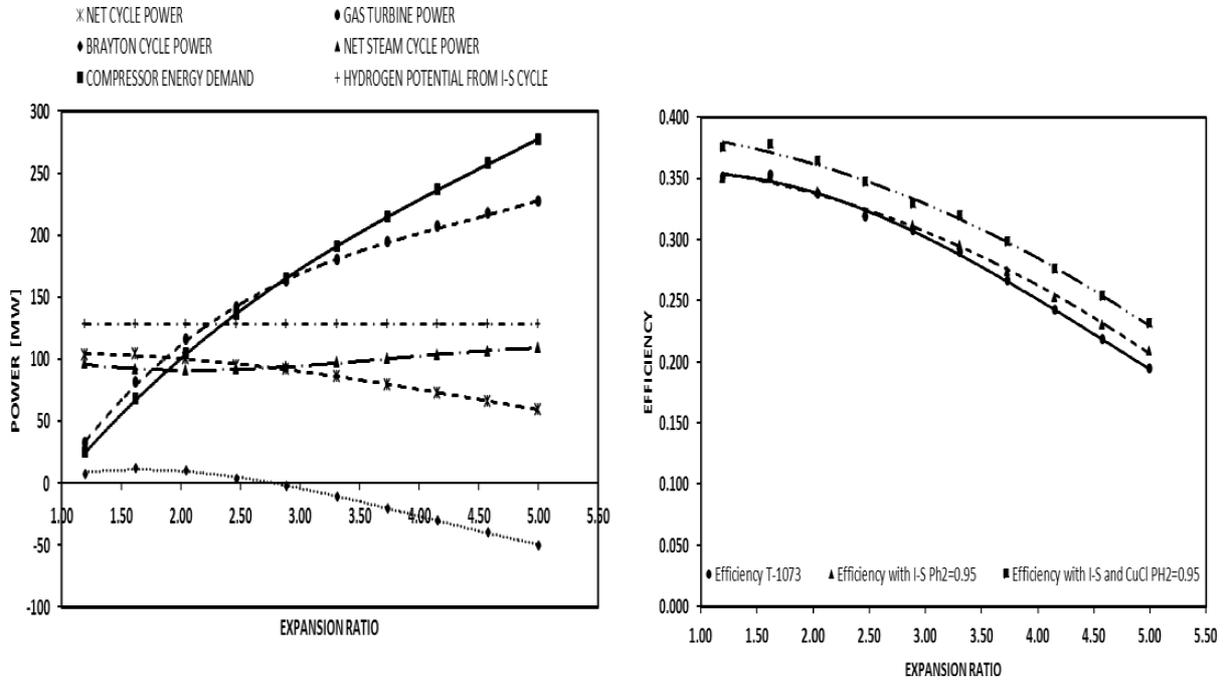
Fig. 5. Thermal power and thermal efficiency versus expansion ratio for the case with simultaneous hydrogen production with I-S and Cu-Cl cycle power,  $P_{H_2} = 30$  MW for I-S cycle and 27 MW for Cu-Cl cycle at the outlet reactor temperature  $T = 1073$  K.
