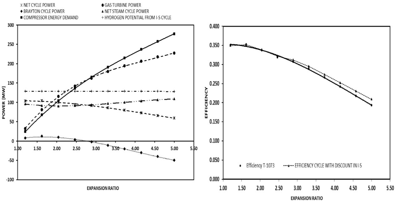
Fig. 4. Power and thermal efficiency versus expansion ratio for the case with hydrogen production using I-S cycle  $P_{H_2} = 30$  MW at the outlet reactor temperature  $T = 1073$  K.
