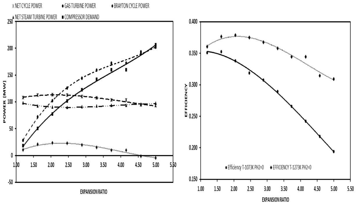
Fig. 6. Power and thermal efficiency at two different outlet reactor temperature  $T = 1073$  K and  $T = 1273$  K for the case without hydrogen production.
