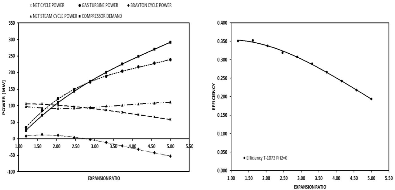
Fig. 3. Power and thermal efficiency versus expansion ratio for the case without hydrogen production at the outlet reactor temperature  $T = 1073$  K.
