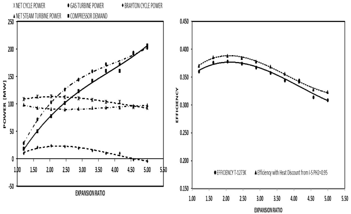
Fig. 7. Power and thermal efficiency at two different outlet reactor temperature  $T = 1073$  K and  $T = 1273$  K for the case with hydrogen production using I-S cycle with the dedicated power  $P_{H_2} = 30$  MW.
