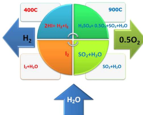
Fig. 2. High-temperature I-S cycle scheme.
