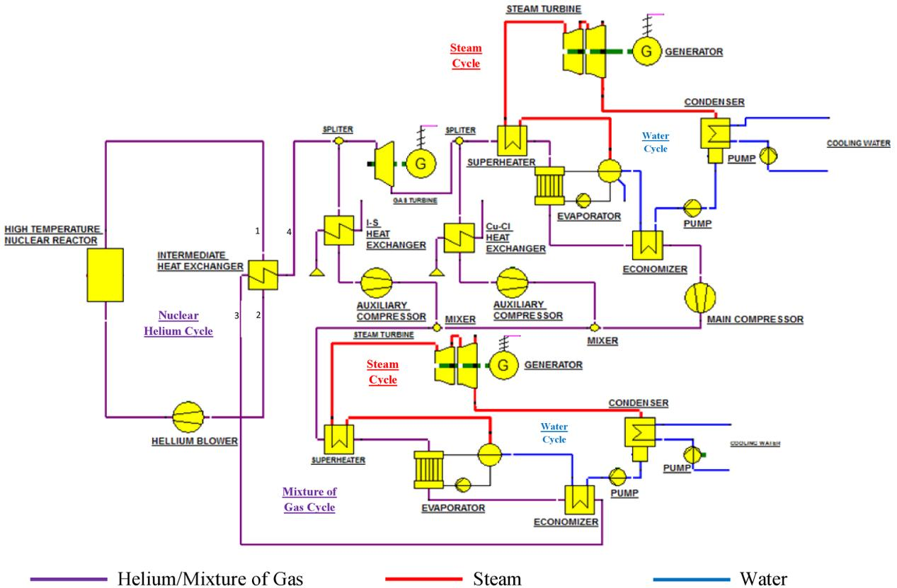
Fig. 1. Gas and steam combined cycle for the HTGR/VTHR with hydrogen production [4].
