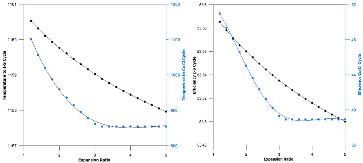
Fig. 9. Outlet temperature and thermal efficiency for I-S and Cu-Cl cycle *versus* expansion ratio for nuclear reactor outlet temperature  $T = 1273$  K.
