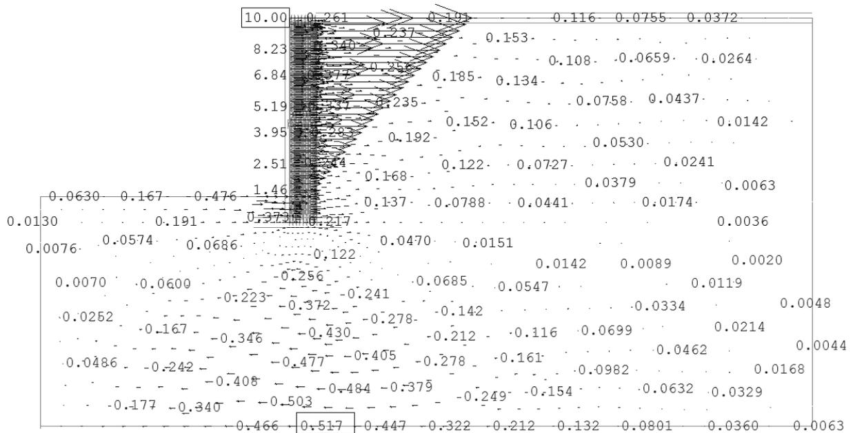
**Fig. 4.** Horizontal displacements with compressive layer [mm] – 3D model results.
