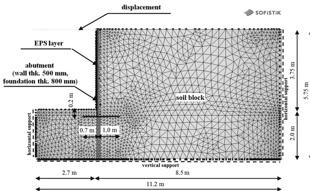
Fig. 1. Visualization of the model.
