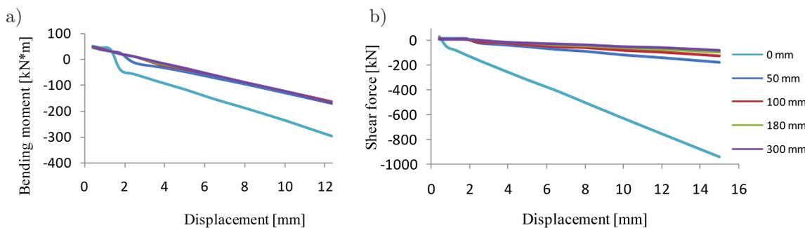
Fig. 5. 2D nonlinear analysis: a) bending moments, b) shear forces.
