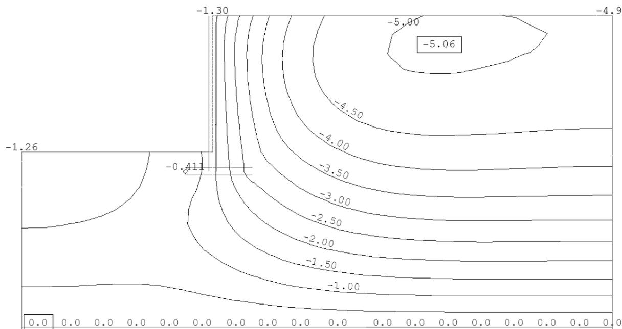
Fig. 8. Vertical displacements with no compressible layer [mm] – 3D model results.
