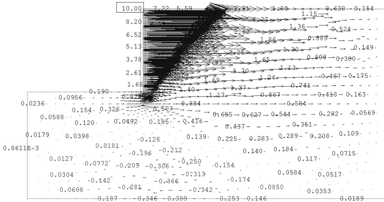
**Fig. 3.** Horizontal displacements without compressive layer [mm] – 3D model results.
