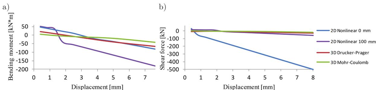
Fig. 6. 3D nonlinear analysis: a) bending moments, b) shear forces.
