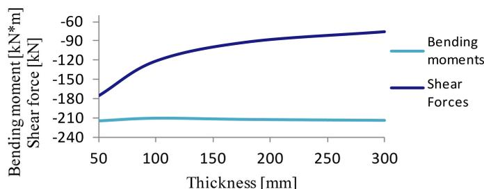
Fig. 7. Influence of thickness of compressible layer – 2D model results.
