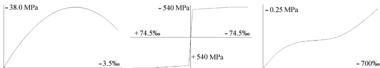
Fig. 2. Stress-strain diagrams (concrete/reinforcement/EPS).
