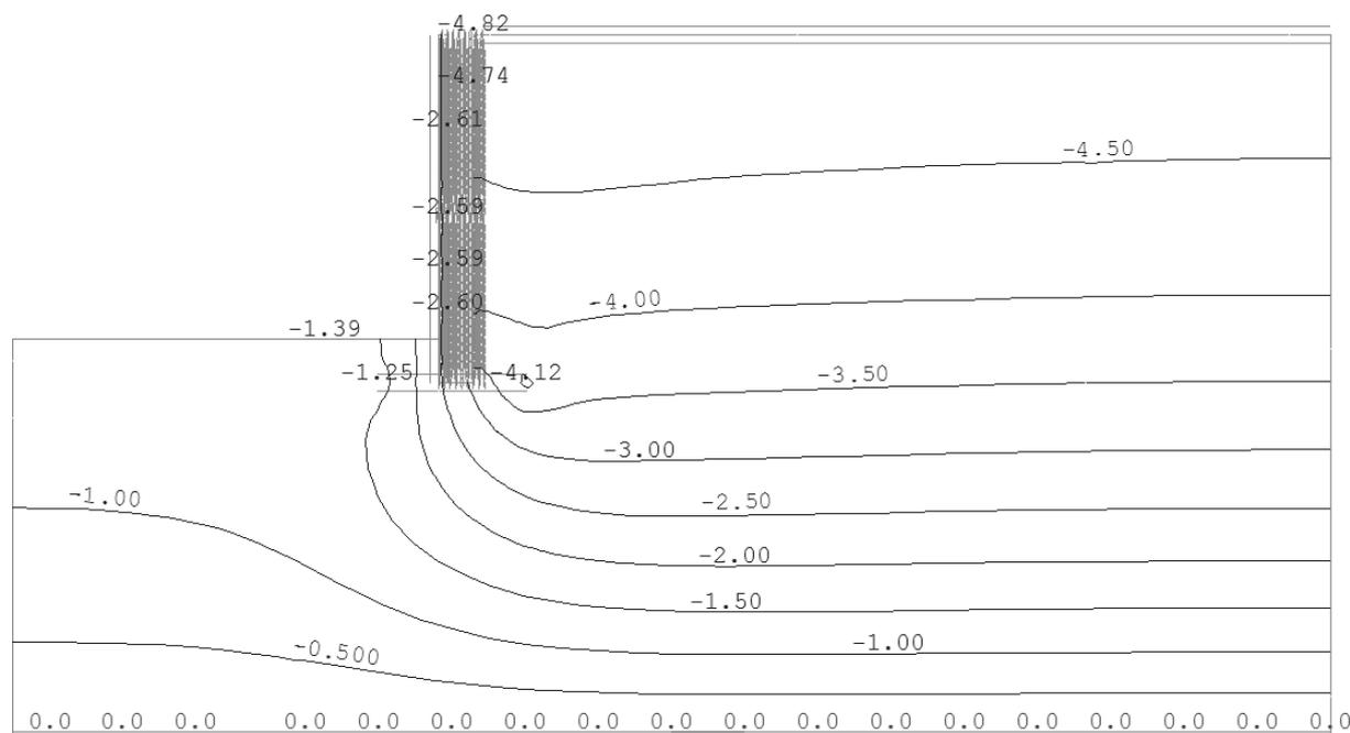
Fig. 9. Vertical displacements with a 100 mm thick compressible layer [mm] – 3D model results.
