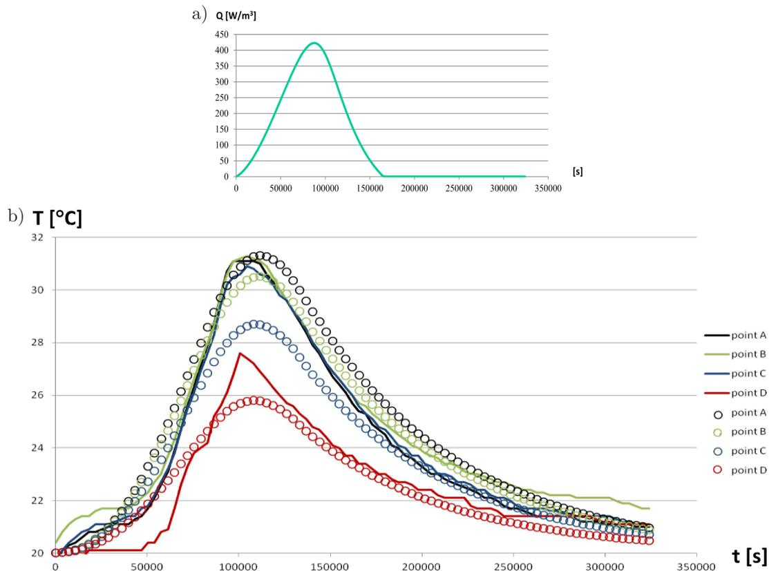
**Fig. 11.** Results for the verification (mixture T51): a) identified function of the heat of the cement hydration, b) comparison between measured and identified temperatures in the sensor points.
