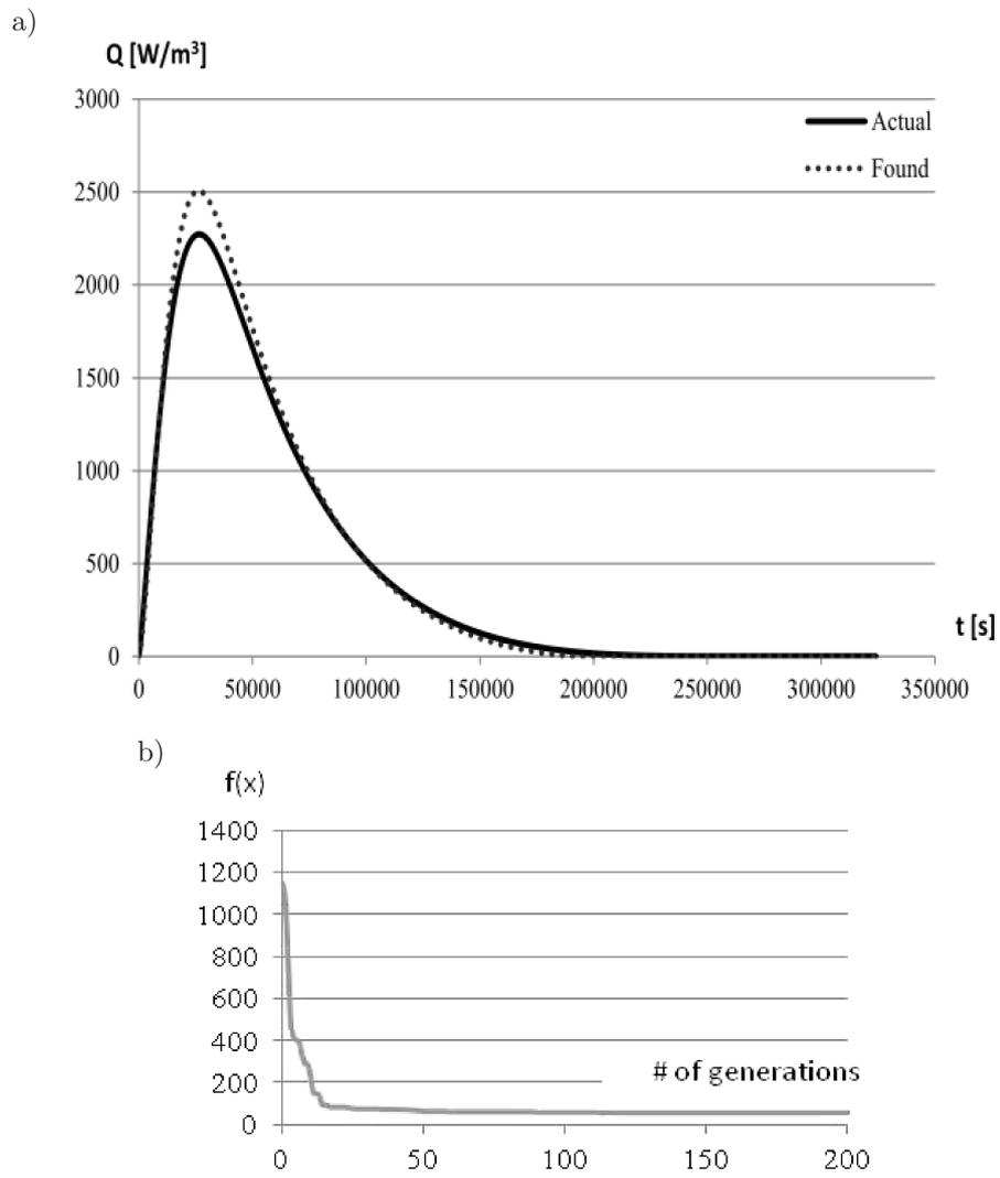
Fig. 6. a) Comparison between actual and identified function of heat of the cement hydration, b) graph of the fitness function value at consecutive generations.
