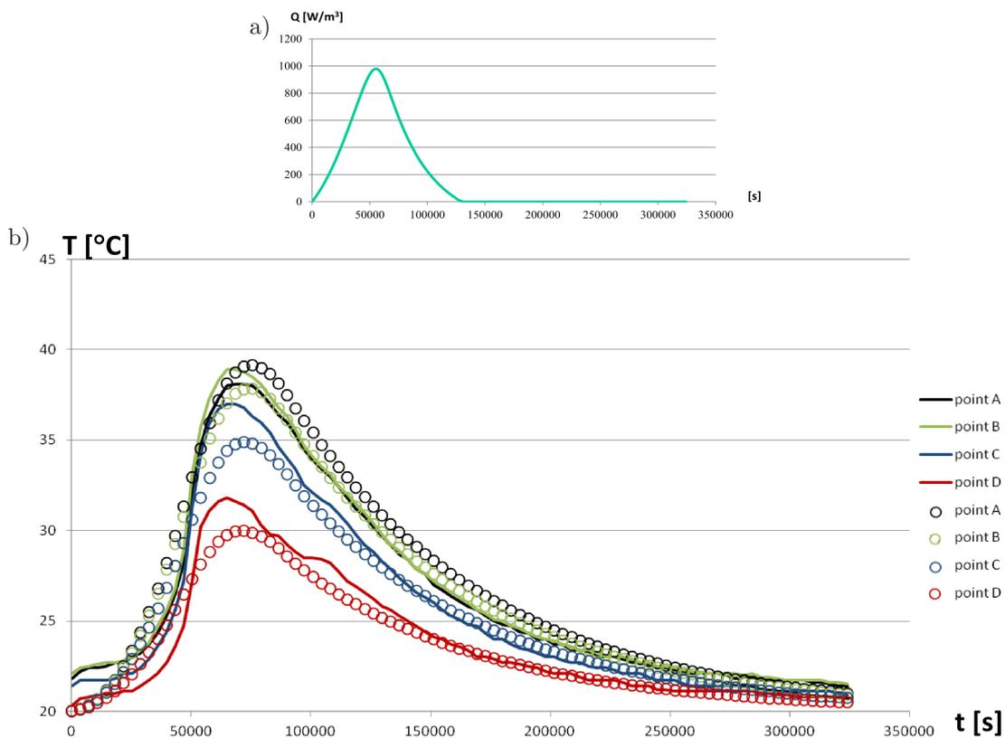
Fig. 9. Results for the verification (mixture T49): a) identified function of the heat of the cement hydration, b) comparison between measured and identified temperatures in the sensor points.
