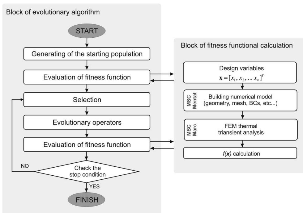
Fig. 5. Flowchart of the identification algorithm.
