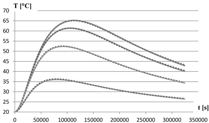
Fig. 7. Results for the verification test. Actual temperature (solid lines) and identified temperatures (dotted lines) in the sensor point of temperature.
