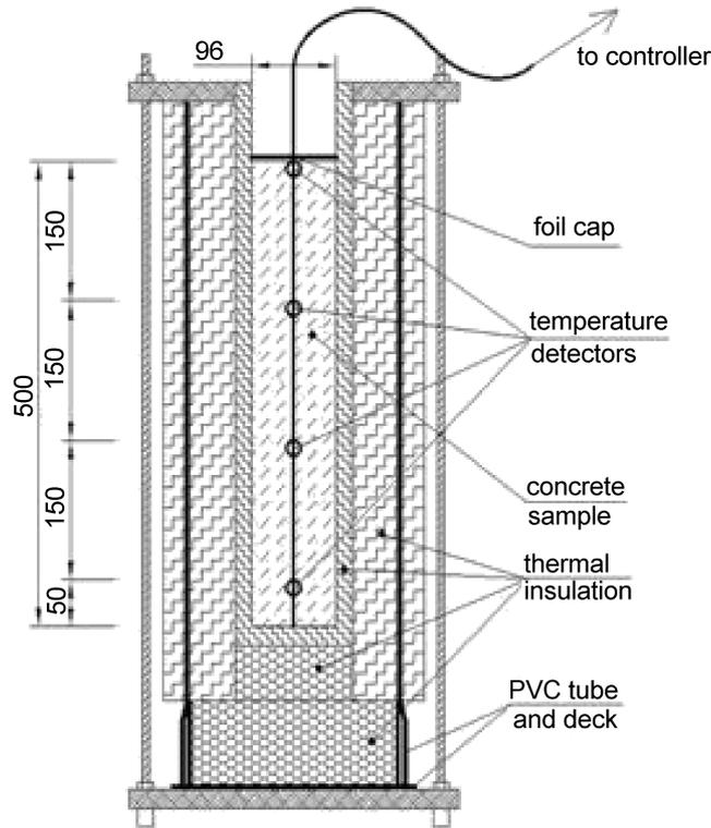
Fig. 2. Model of the mould.
