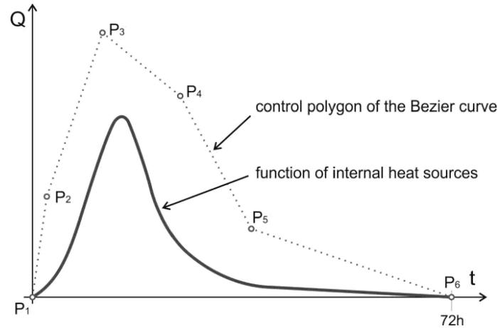
Fig. 1. The method of parameterization of the heat of cement hydration.
