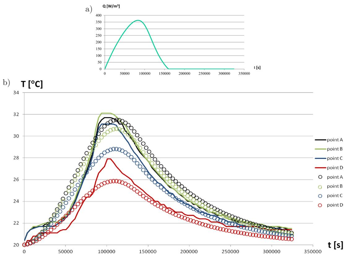
Fig. 10. Results for the verification (mixture T50): a) identified function of the heat of the cement hydration, b) comparison between measured and identified temperatures in the sensor points.
