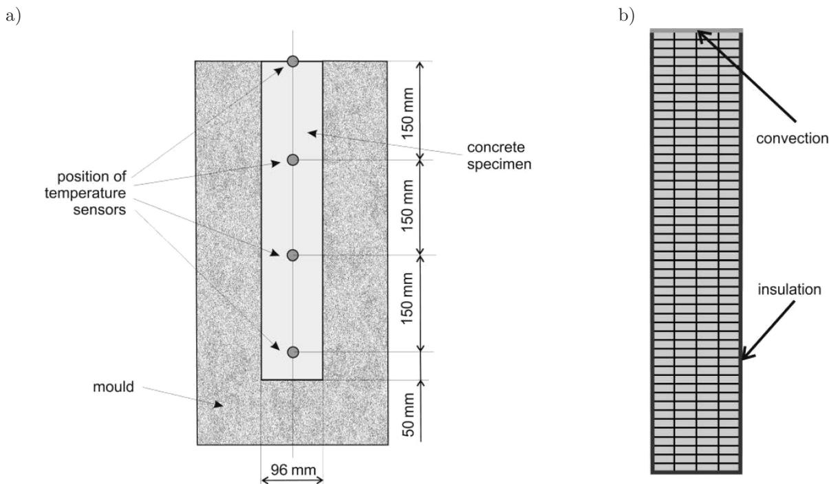
Fig. 4. a) Model of concrete specimen, b) two-dimensional (2D) numerical model with boundary conditions.
