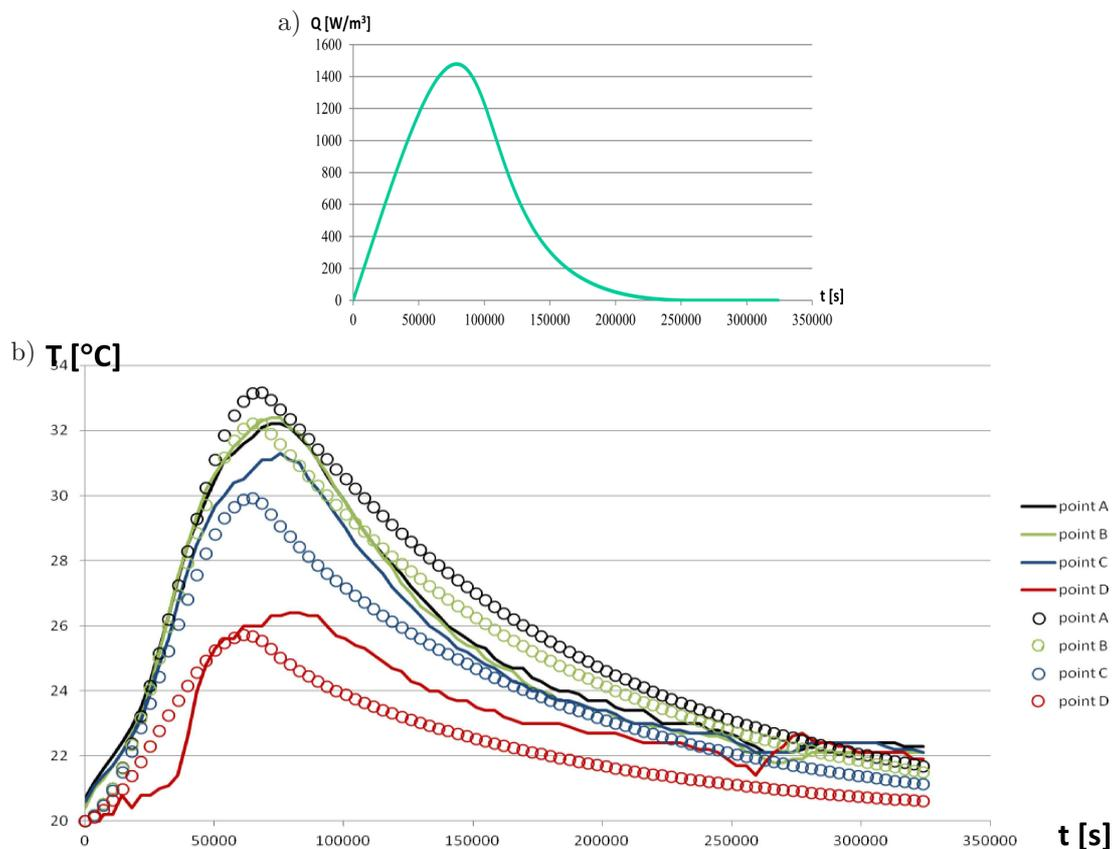
**Fig. 8.** Results for the verification (mixture T26): a) identified function of the heat of the cement hydration, b) comparison between measured and identified temperatures in the sensor points.
