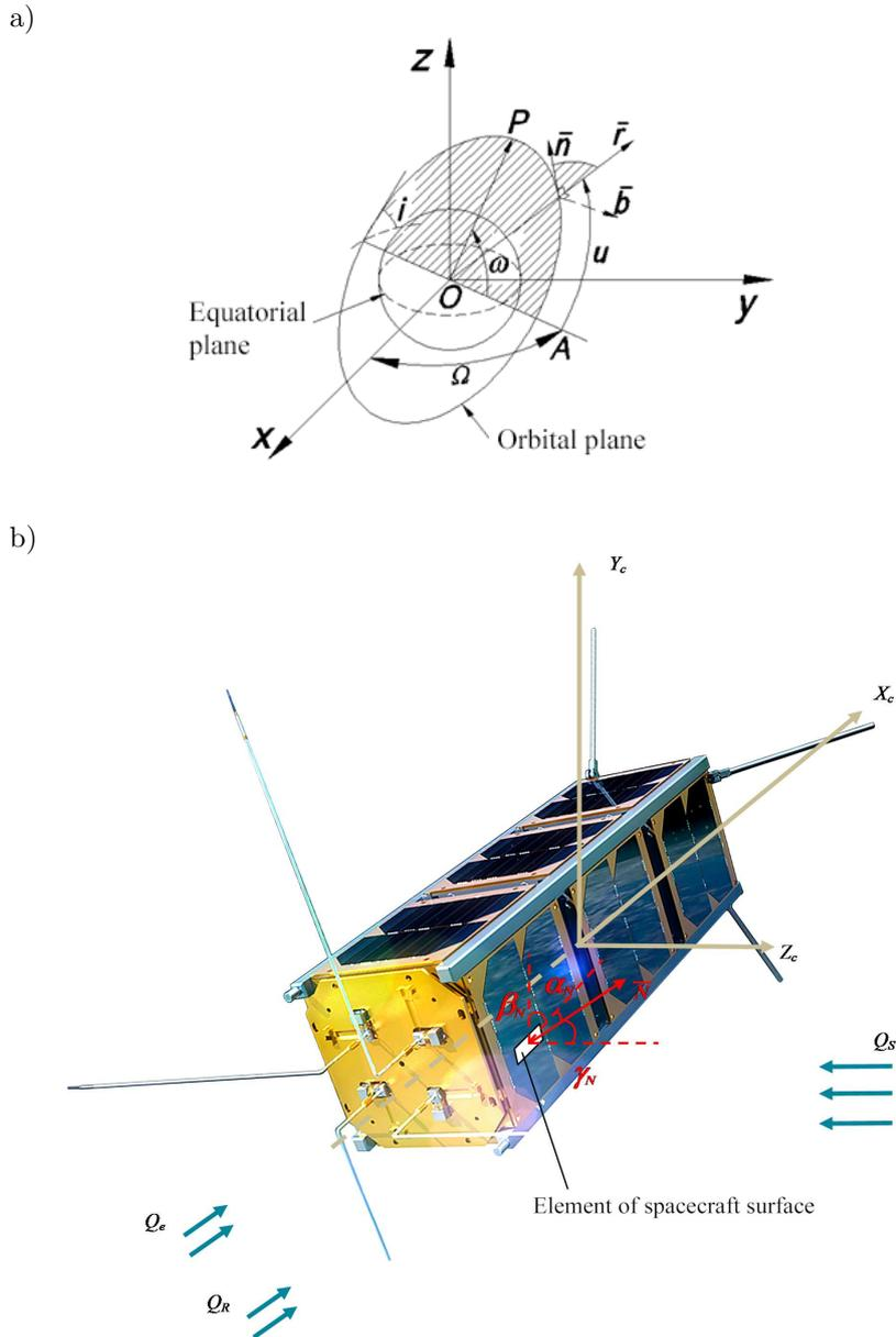
**Fig. 1.** The orientation of the surface element: a) in the equatorial and orbital coordinate systems, b) in the coordinate system associated with the spacecraft.
