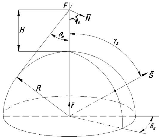
Fig. 2. The main parameters for angular coefficients calculation.
