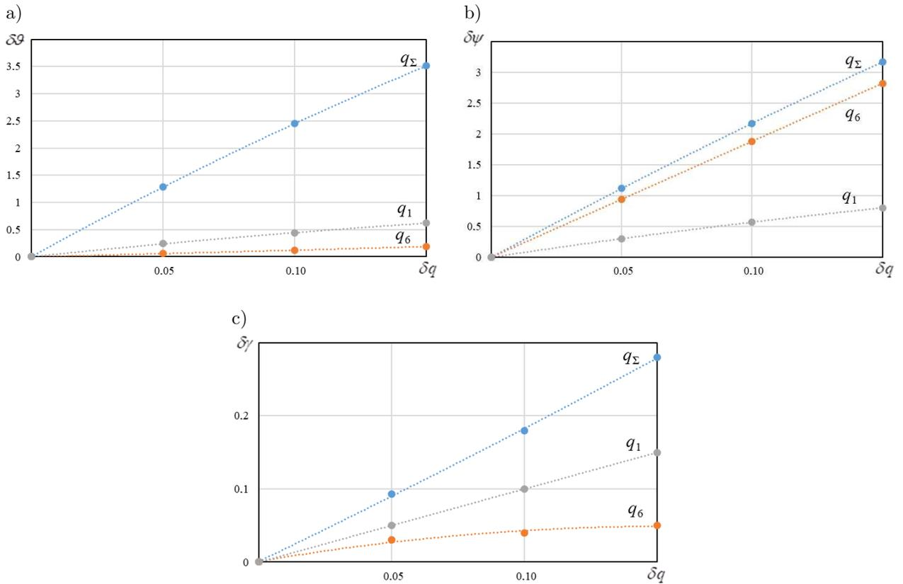
**Fig. 10.** Errors of recovery of the angular position of the spacecraft in the presence of heat leaks on the: a) 3rd, b) 6th and c) all six sensors simultaneously.
