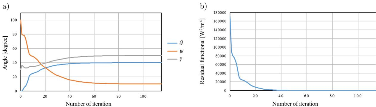
**Fig. 9.** a) Inverse problems solution results for the “exact” values  $\vartheta = 40^\circ$ ,  $\psi = 10^\circ$ ,  $\gamma = 50^\circ$ , b) the initial approximation for the conjugate gradient method is:  $\vartheta = 0^\circ$ ,  $\psi = 100^\circ$ ,  $\gamma = 30^\circ$ .
