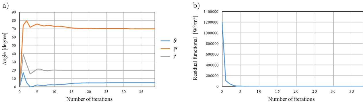
Fig. 6. a) Inverse problems solution for the "exact" values  $\vartheta = 5^\circ$ ,  $\psi = 70^\circ$ ,  $\gamma = 20^\circ$ , b) the initial approximation for the conjugate gradient method is:  $\vartheta = 0^\circ$ ,  $\psi = 0^\circ$ ,  $\gamma = 0^\circ$ .
