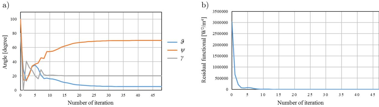
**Fig. 7.** a) Inverse problems solution for the “exact” values  $\vartheta = 5^\circ$ ,  $\psi = 70^\circ$ ,  $\gamma = 20^\circ$ , b) the initial approximation for the conjugate gradient method is:  $\vartheta = 80^\circ$ ,  $\psi = 100^\circ$ ,  $\gamma = 75^\circ$ .
