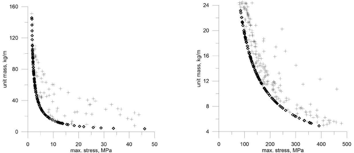
Fig. 5. The Pareto front at the background of initial population – beam optimization example (left), cryogenic pipe optimization (right).
