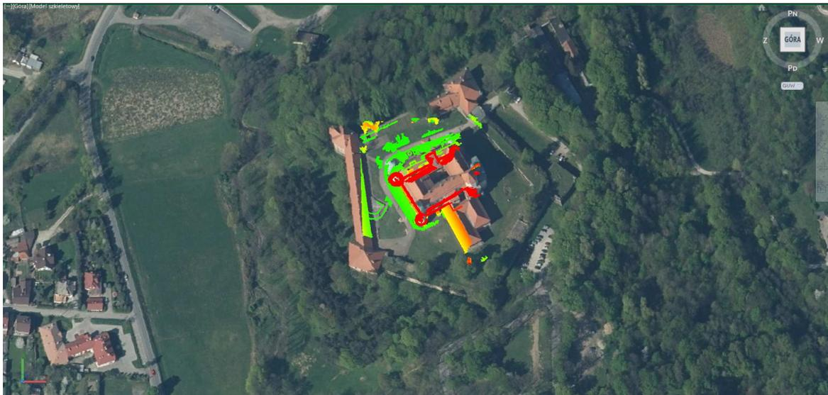
**Fig. 7.** Digital model embedded in the orthophotomap to check the correctness of its proportions.
