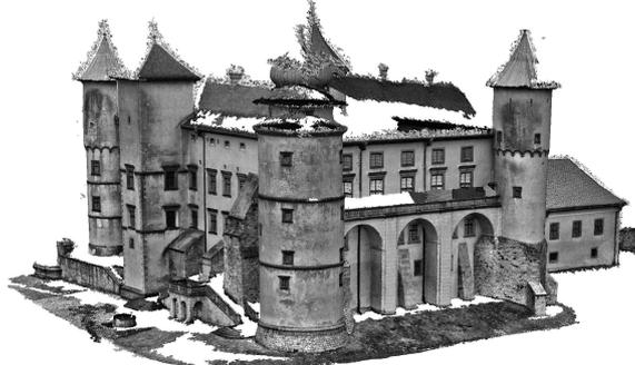
**Fig. 5.** Reconstruction performed with the use of images after adaptive histogram equalizing.
