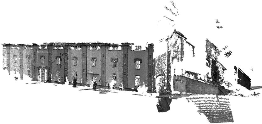
**Fig. 10.** Reconstruction performed with the use of images after histogram stretching.
