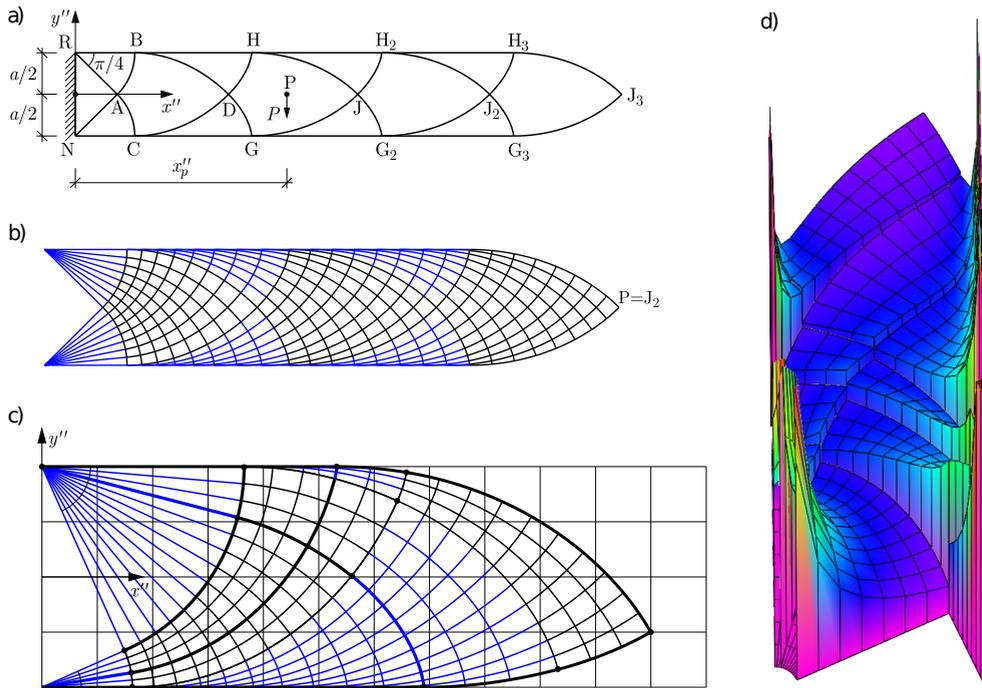
FIG. 3. Optimal Michell cantilever transmitting point load to straight support: a) arrangement of the regions of kinematic division for  $\sigma_T = \sigma_C$ ; b) geometry of Hencky net for  $\sigma_T = \sigma_C$ ; c) arrangement of regions of kinematic and static division for  $\sigma_T = 5\sigma_C$ ; d) the alternate thickness distribution of the cantilever for  $\sigma_T = 5\sigma_C$ .
