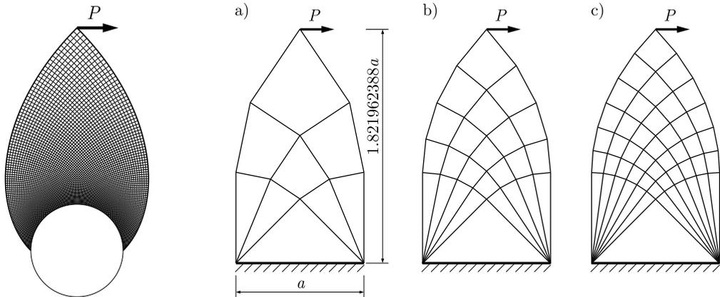
FIG. 2. Left: Michell cantilever transmitting point load to circular support (case of equal permissible stresses in tension and compression); right: three subsequent suboptimal trusses transmitting given force to a straight support: a)  $V_r = 6.1605$ , b)  $V_r = 6.0953$ , c)  $V_r = 6.0835$ , where  $V_r = V/V_0$ ,  $V_0 = Pa/\sigma_0$ ,  $\sigma_0$  being the permissible stress.
