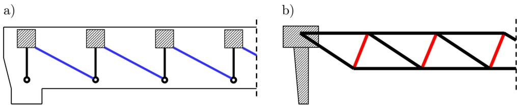
FIG. 11. a) The initial design of the Spodek roof by Waclaw Zalewski, b) the final design of the Spodek roof (based on drawings by M. Pelczarski [30]).
