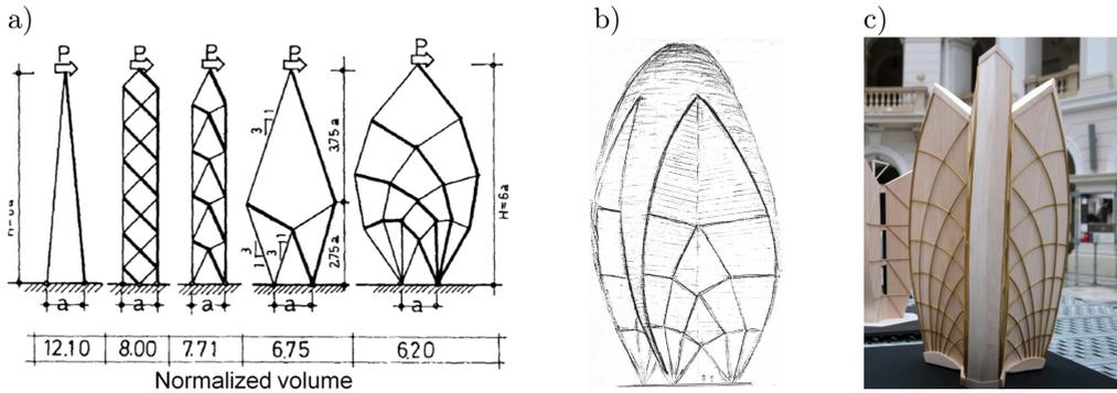
FIG. 4. a) Comparison of various topologies by Zalewski and Zabłocki [21]; b) sketch of “tulip-like building” (source: <http://www.wz-structure.org/#/unbuilt/>); c) wooden model of “wingy building” (source: <https://www.pw.edu.pl/Uczelnia/Materialy-promocyjne/Galeria/Konstrukcje-Waclawa-Zalewskiego-fotorelacja>).
