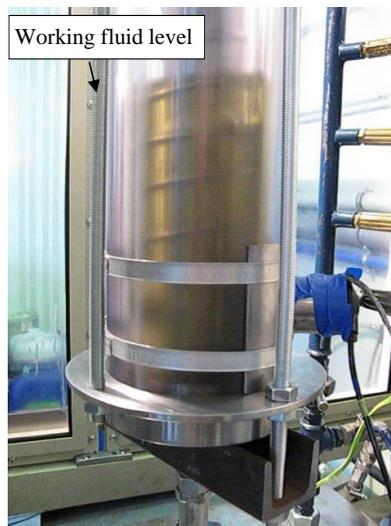
FIG. 2. A transparent shock absorber installed in the test rig.
