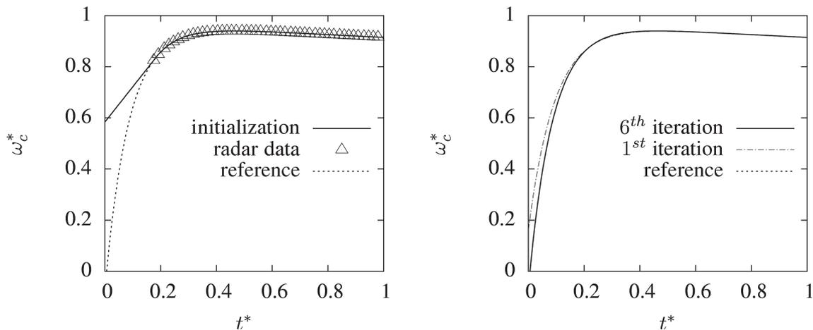
Fig. 4. Reconstruction of the roll rate parameter  $\omega_c$  using only radar data.
