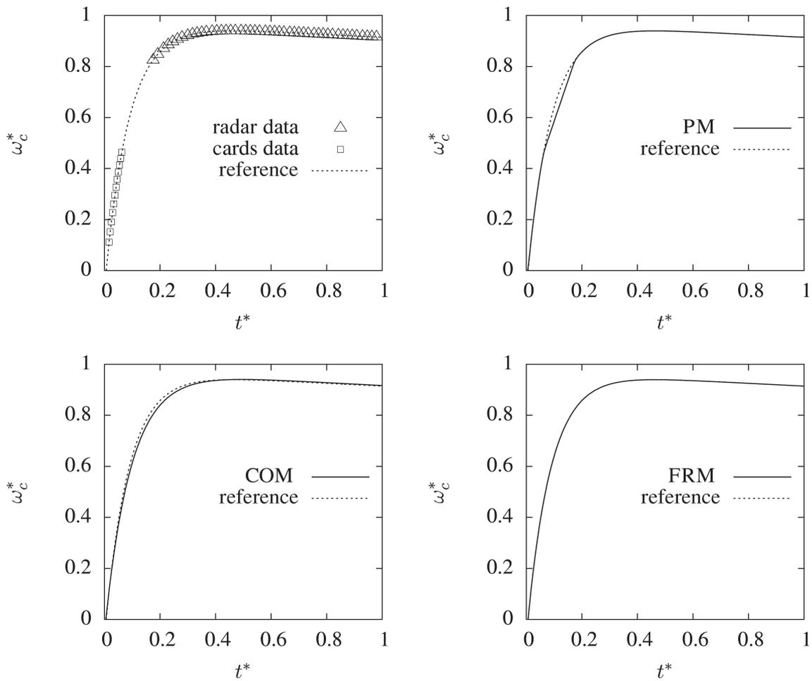
**Fig. 2.** Reconstruction of the roll rate parameter  $\omega_c$  using simulated non-noised yaw cards and radar data.
