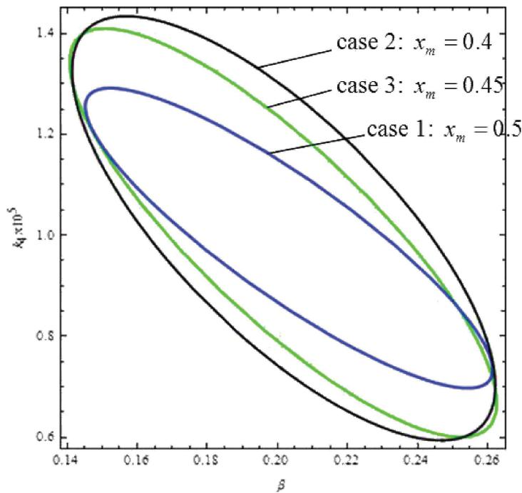
**Fig. 5.** Direct comparison of the elliptic joint confidence regions for  $\beta$  and  $K_4$  estimated in cases 1, 2 and 3.
