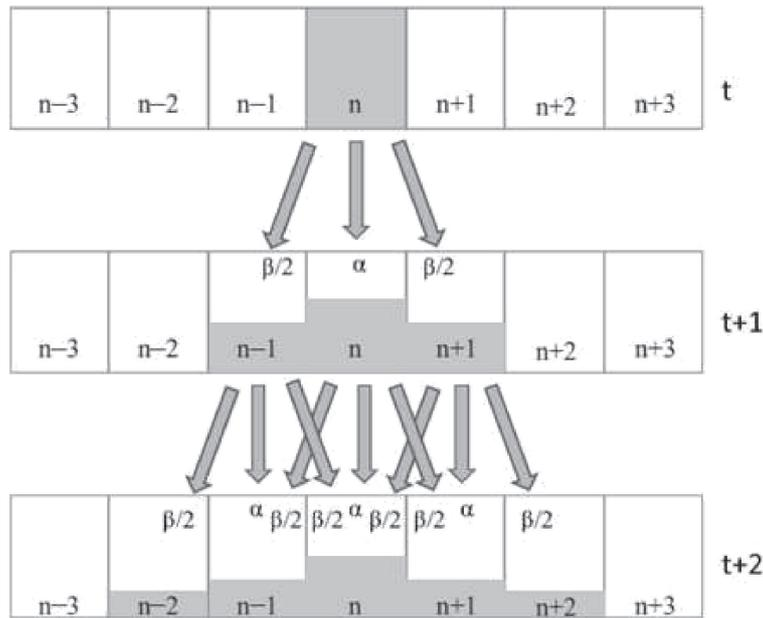
**Fig. 1.** Schematic representation of the symmetric distribution with retention  $\alpha = (\beta - 1)$ .
