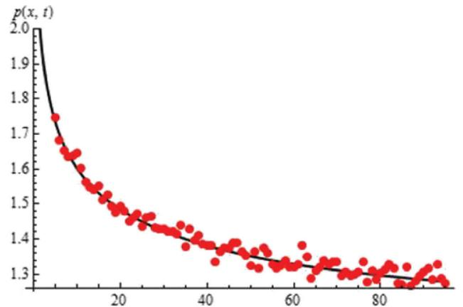
**Fig. 3.** Simulated experimental data (red dots) for transient measurements of a sensor located at  $x = 0.5$ . The black curve shows the numerical solution employed to simulate the experimental data.
