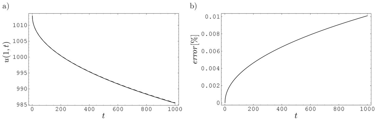
**Fig. 1.** Distribution of temperature  $u(x, t)$  for  $x = 1$  obtained using ACO algorithm for 2% error of input data (a): solid line – exact solution, dashed line – approximated values) and error of this approximation (b).
