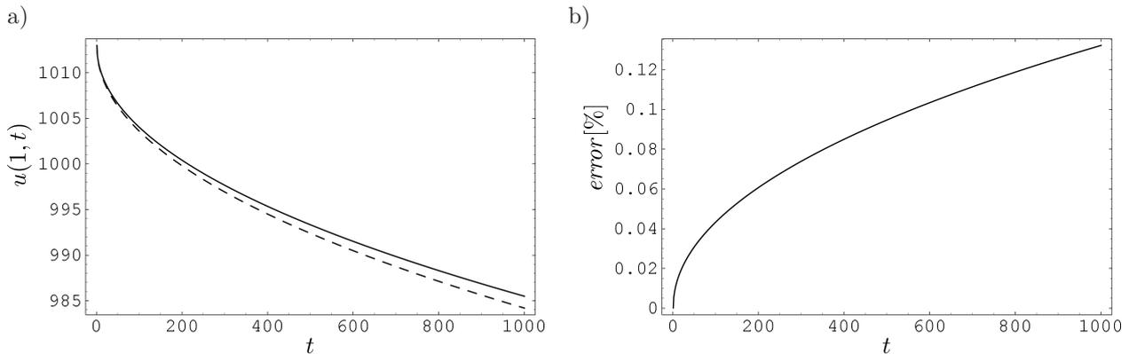
**Fig. 4.** Distribution of temperature  $u(x, t)$  for  $x = 1$  obtained using ABC algorithm for 5% error of input data (a): solid line – exact solution, dashed line – approximated values) and error of this approximation (b).
