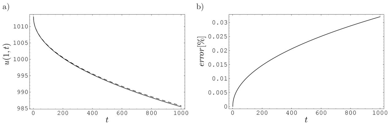
**Fig. 2.** Distribution of temperature  $u(x, t)$  for  $x = 1$  obtained using ABC algorithm for 2% error of input data (a): solid line – exact solution, dashed line – approximated values) and error of this approximation (b).
