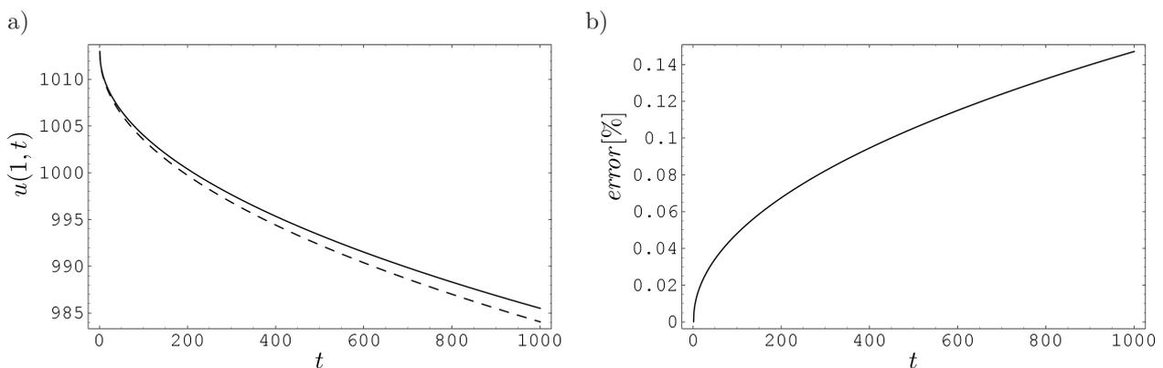
**Fig. 3.** Distribution of temperature  $u(x, t)$  for  $x = 1$  obtained using ACO algorithm for 5% error of input data (a): solid line – exact solution, dashed line – approximated values) and error of this approximation (b).
